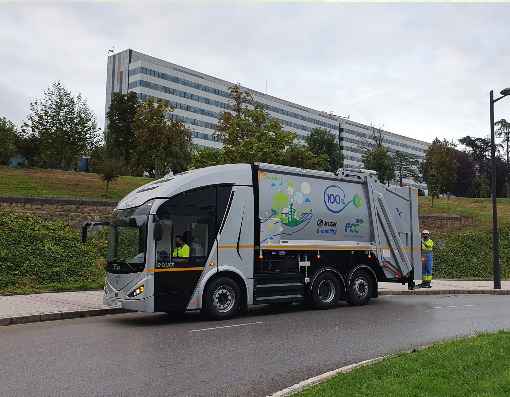
Ie-Urban truck: rear-loading electric collection vehicle developed on FCC Environment's e-mobility platform.
